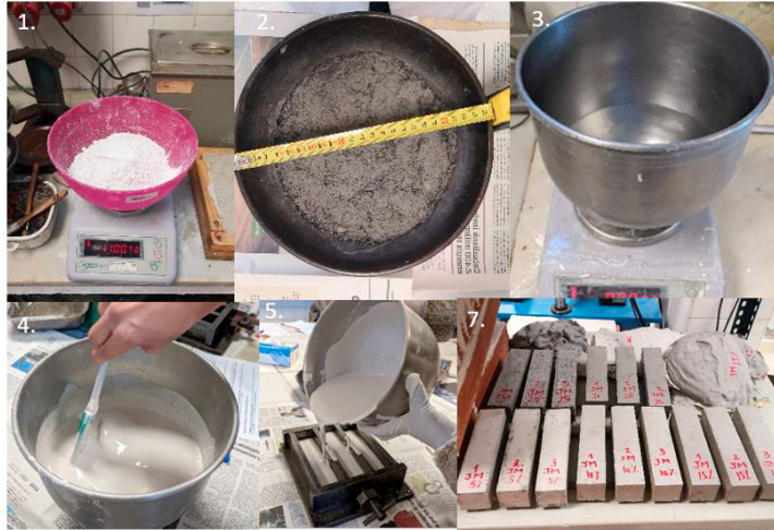
Fig. 1. Samples preparation according EN 13279-2.
