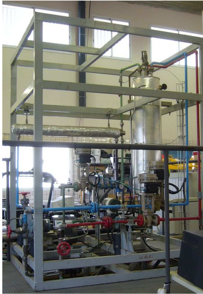
Figure 3.1: Pilot plant used to study different model-based predictive control strategies.
