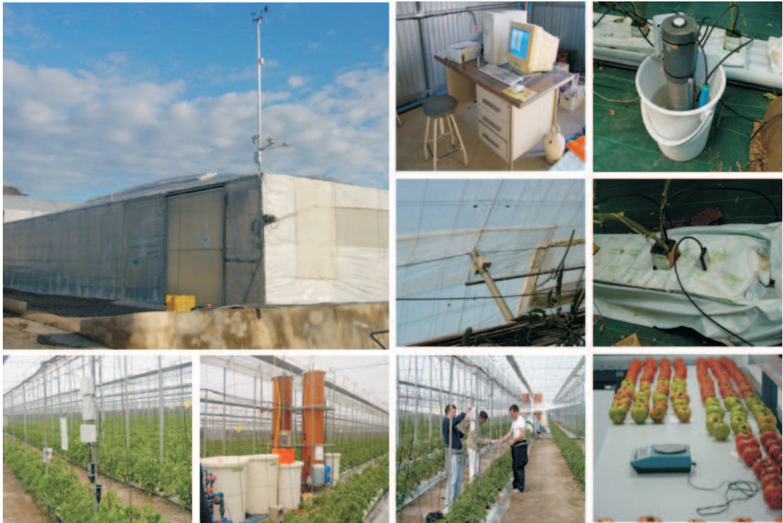
Figure 3.23: Exterior view of the used experimental greenhouse and photos of the control and monitoring system as well as some of the installed sensors in the interior of the greenhouse.
