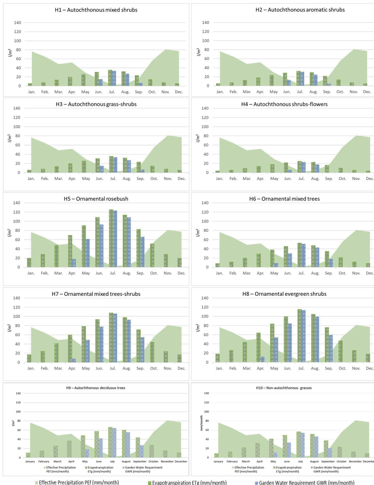
Fig. 5. Rain patterns and water necessities of the 10 hydro-zones in the garden.
