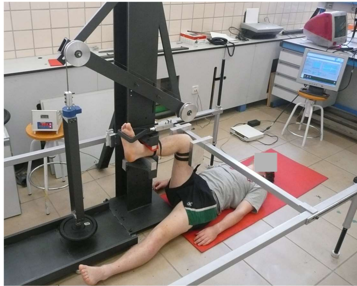
Fig. 7. Global view of the experimental apparatus based on the measurement of the rotation of the foot around the ankle articulation.
