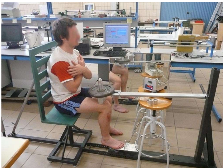
Fig. 2. Global view of the experimental apparatus based on the measurement of lower leg vertical displacements.
