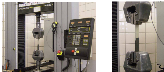
Fig. 4 - Testing of the samples in shear by a tensile loading.
