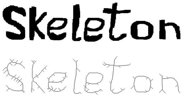
Fig. 3 A hand-written word and its skeletonization. Image borrowed from [49]
