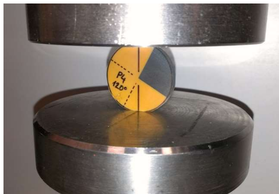
Figure 3.- Test of one specimen containing the bimaterial corner in compression to obtain the failure envelope.
