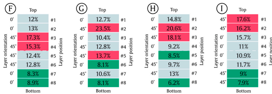
Fig. 23. Energy dissipated by each layer due to intralaminar damage for stacking sequences F, G, H, and I.
