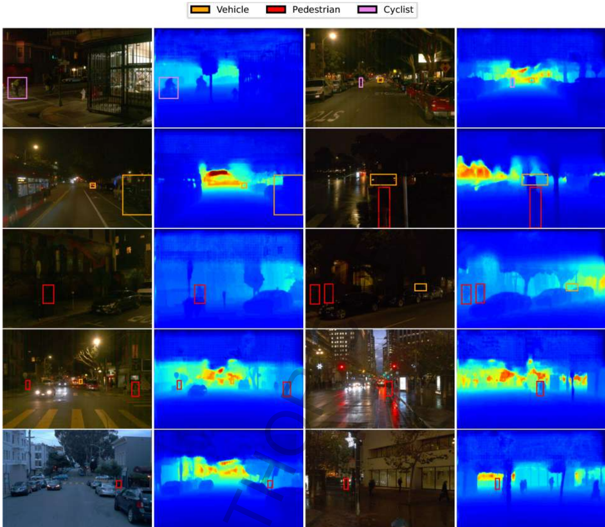
Fig. 5. Typical examples illustrating the advantages of the proposed dual-modal detection approach. The highlighted objects are detected by our RGB-LDCNet fusion network, but the RGB-only models fail to detect them. For each scene, the camera images and the dense LDCNet depth maps are displayed.
