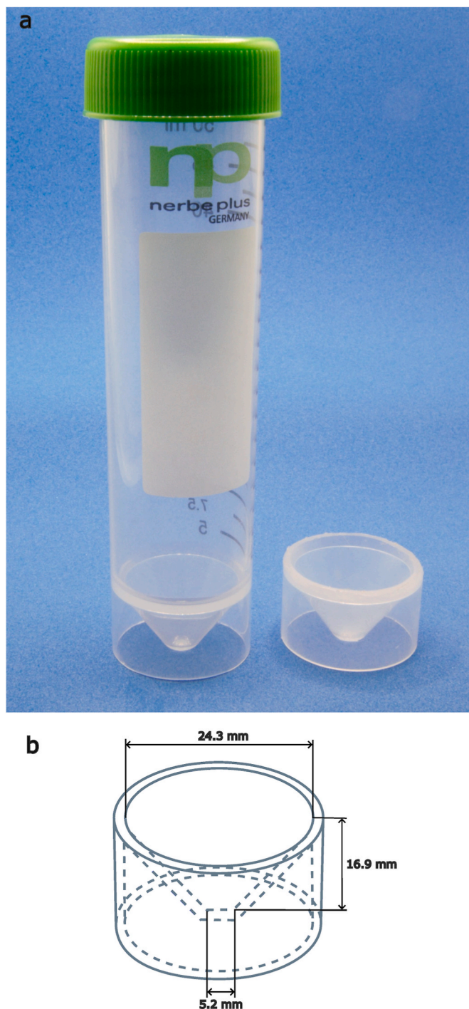
Fig. 1. Description of the sample holder capsule. (a) Initial polypropylene centrifuge tube and sample holder capsule made from it. (b) Dimensions of the sample holder capsule.
