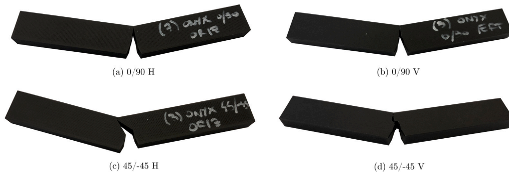
Fig. 4. Tested SENB specimens for the different configurations: (a) 0/90 Horizontal (b) 0/90 Vertical (c) 45/-45 Horizontal (d) 45/-45 Vertical.
