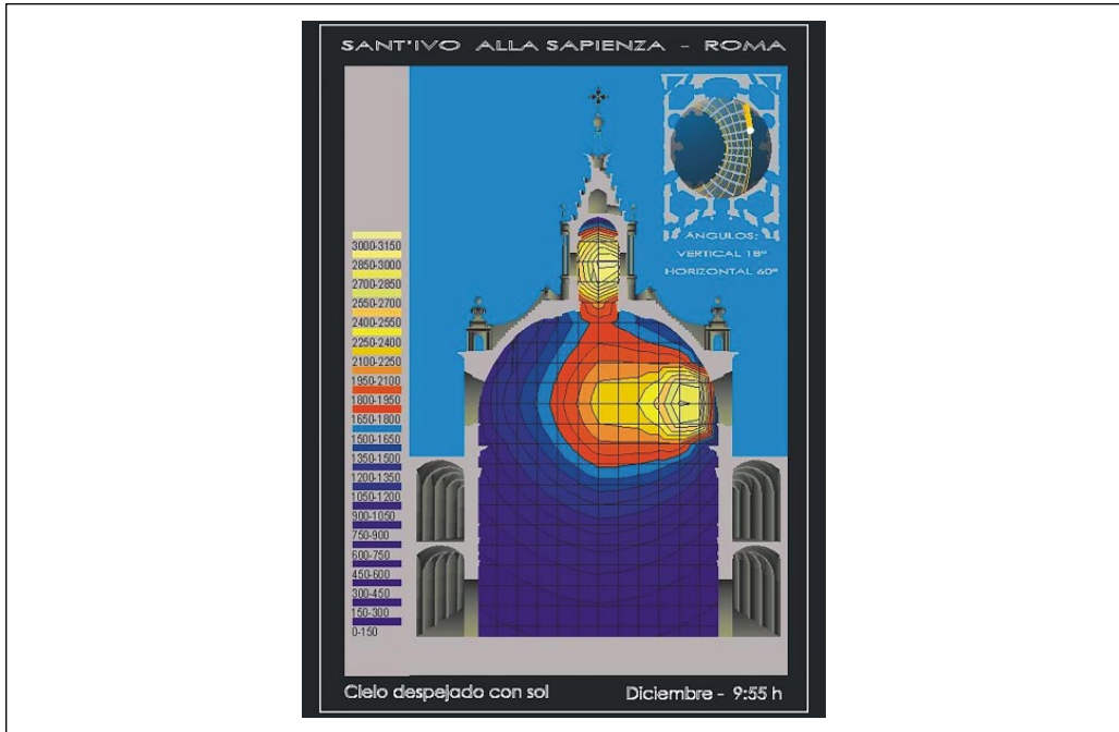
Figure 5. Excerpt from the simulation sequence of the interior of the church of Sant'Ivo, December at 9:45 hours (section).
