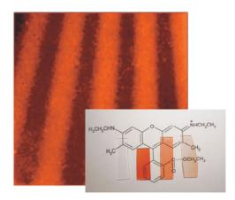
Luminescent nanocomposites containing Rhodamine 6G laser dye molecules have been deposited by remote microwave plasma polymerization. The synthesis is tailored to avoid dye aggregation in order to enhance the fluorescent emission and to control the optical properties. Nanometric films deposited by this novel methodology are intensely absorbent and fluorescent. Micrometric patterns can be generated by plasma etching using a shadow mask.
