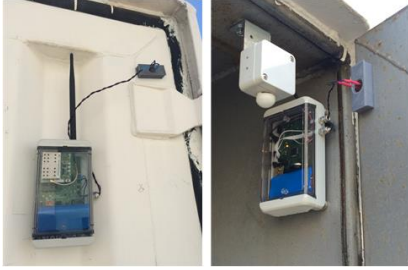
Figure 4. Transponder controller outside the container (left) and acquisition board inside the container (right)
