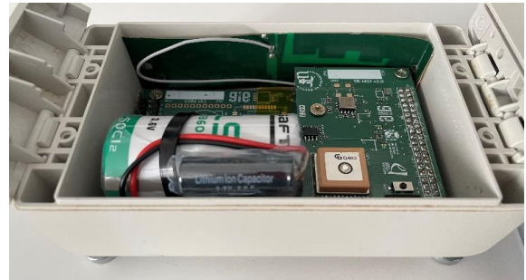
Fig. 3. Assembled Node (CoreBoard + SensorBoard + Antenna + Battery + Enclosure)
