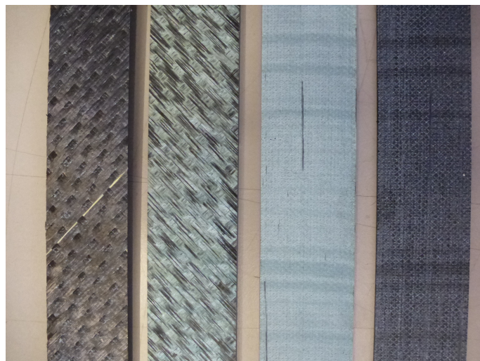
Figure 7: Fracture surfaces obtained for the fabric (left) and tape (right) case in the HDP test.
