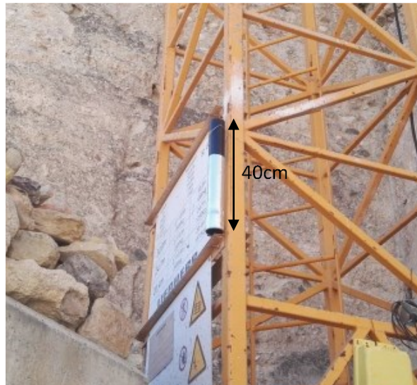
Figure 7. Sensors for monitoring outdoor temperature. Source: J. Arco
