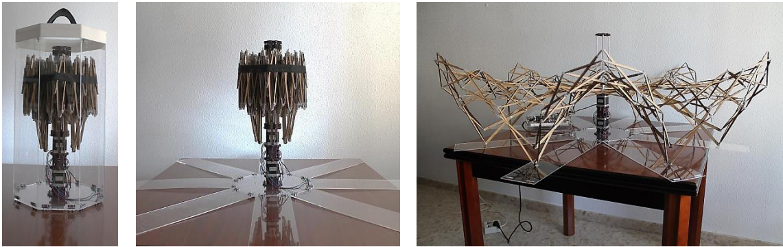
148 149 Fig. 8. Deployment process of the geometry “Los Manantiales” in Xochimilco, Mexico (Author: 150 Félix Candela).
