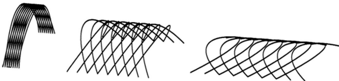
116 117 Fig. 5. Deployment process of the structure designed by Félix Escrig Pallarés and Jose Sánchez- 118 Sanchez
