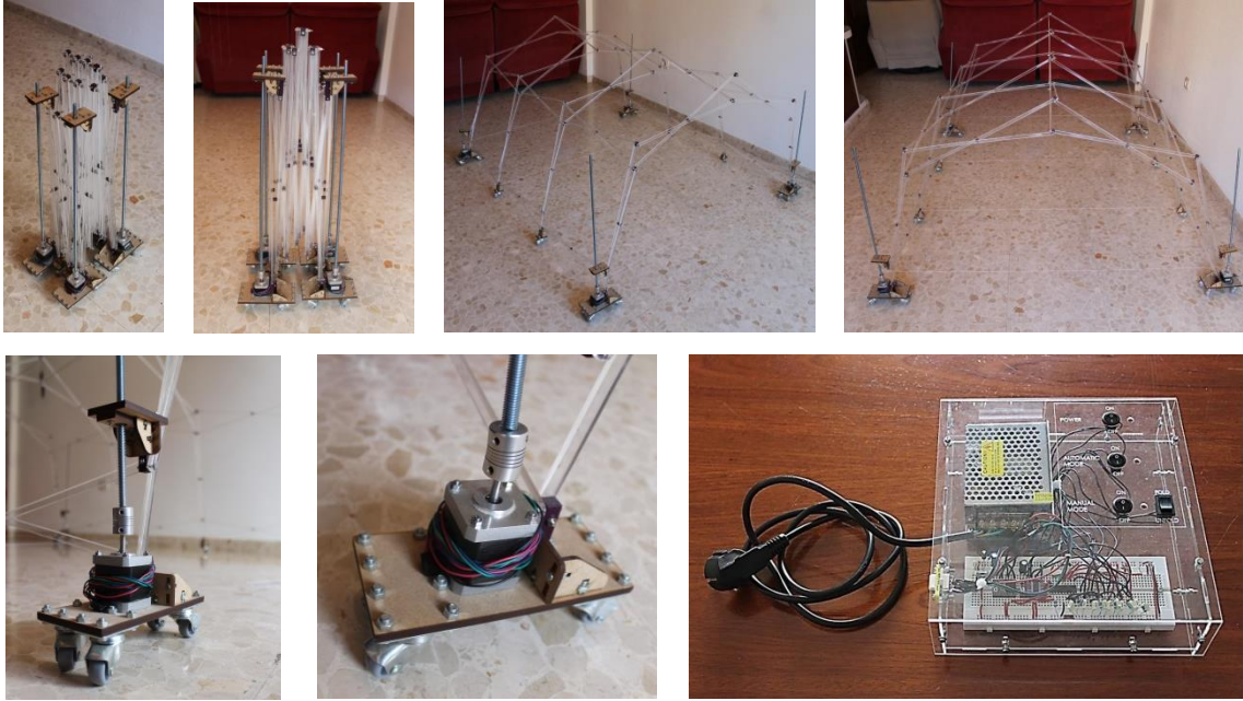
376 377 Fig. 15. Folded and unfolded positions of the built structure using stepper motors in the focal 378 directions and the electronics required.
