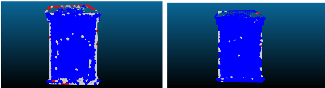
425 426 Figure 14. (a) Test G; (b) Test H. Classification through the CANUPO plug-in.
