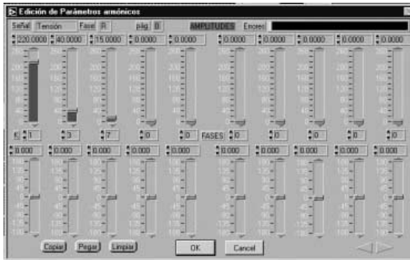
Fig. 2. Parameter settings showing the harmonic content of the voltage waveform
