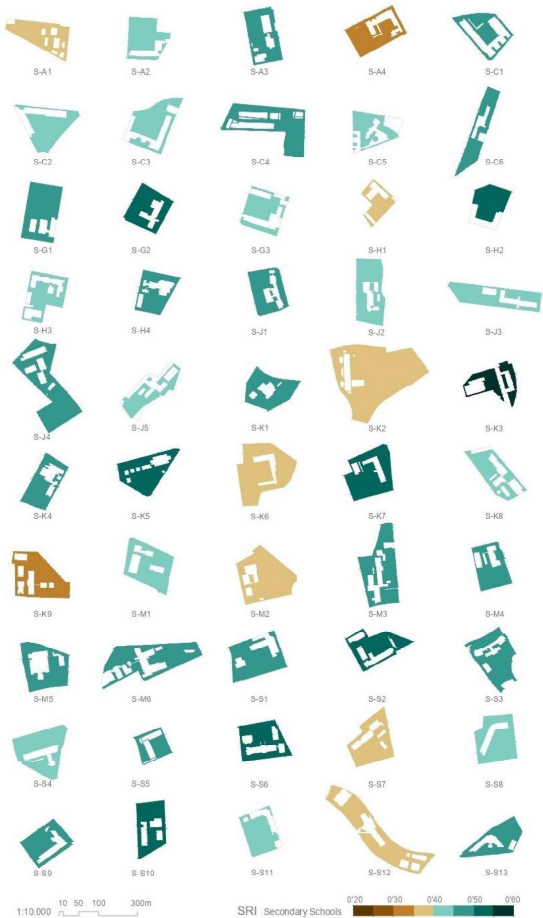
Figure 9. Outdoor area with respect to Secondary school buildings and mean SRI value on a scale.
