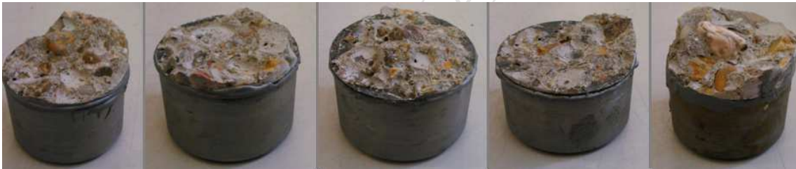
Figure 21. Failure of the grinder surface-treated, infusion manufactured shear torsion coupons
