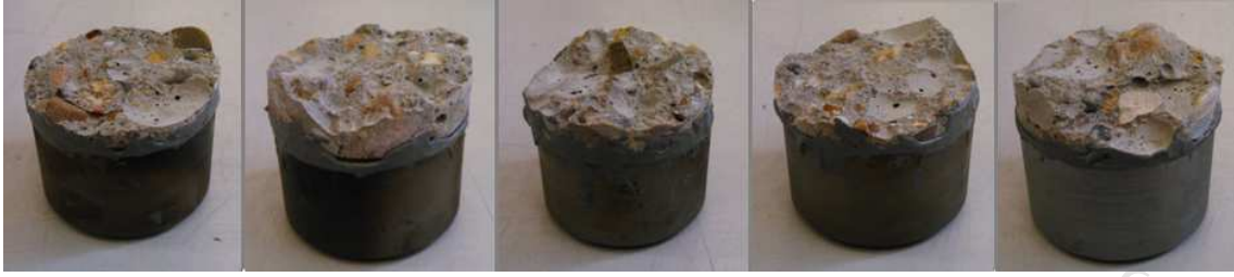
Figure 19. Failure of the grinder surface-treated, infusion manufactured pull off coupons
