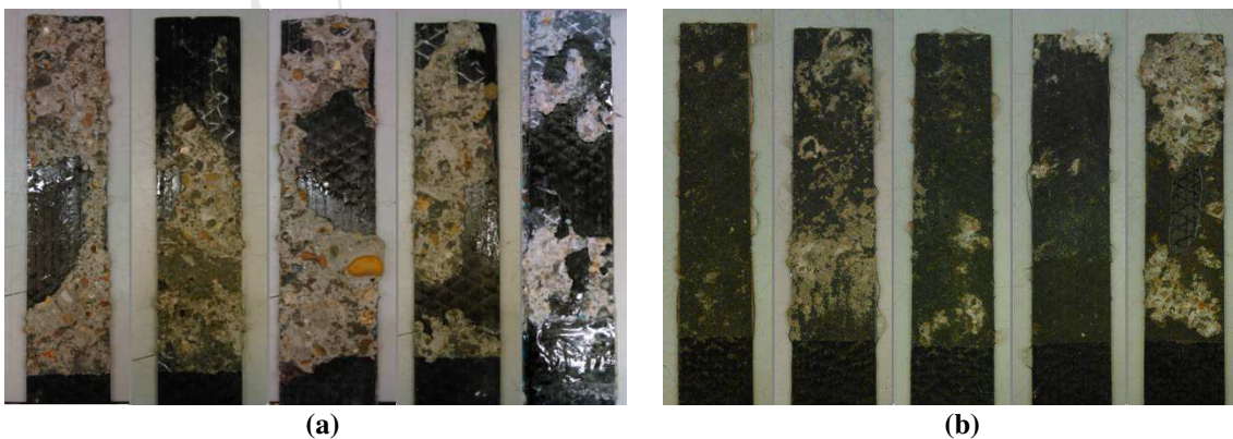
Figure 18. Composite failure surfaces after the lap shear test for (a) grinder surface-treated coupons and (b) grit sandpaper surface-treated coupons
