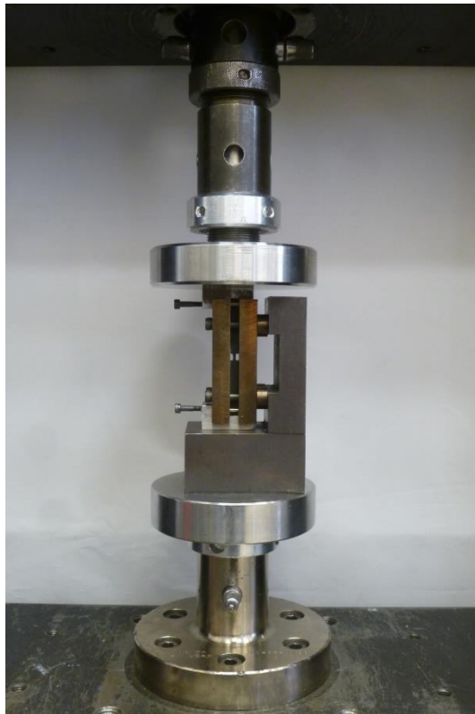
Figure 4. Compressive test set-up.
