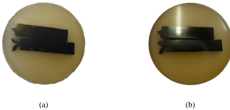
Figure 6. Sample (a) before polishing (b) after polishing.
