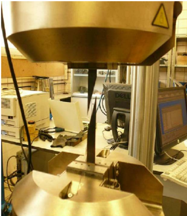
Figure 4. View of a dynamic test for 15° orientation angle of the fibres.
