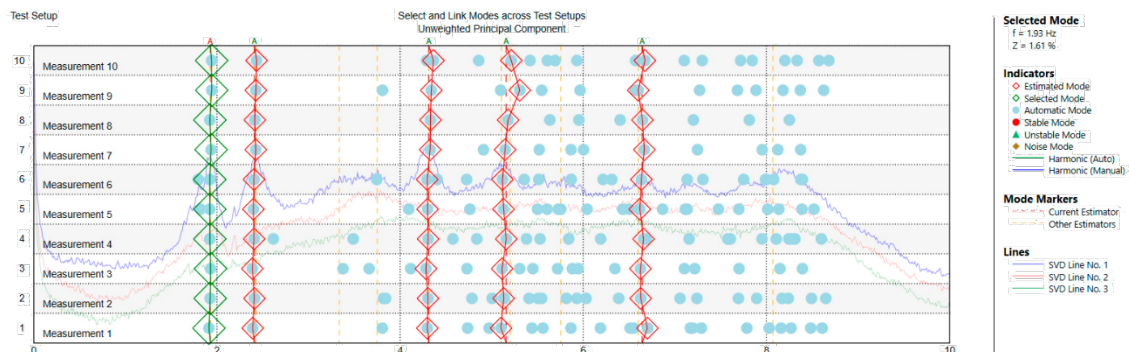
Figure 14. Identification of Modal Parameters in the stochastic subspace
