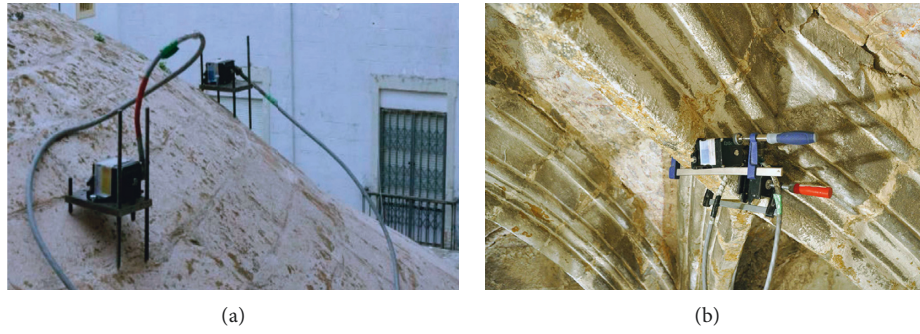
FIGURE 11: Accelerometers on the extrados and the intrados of the vault.
