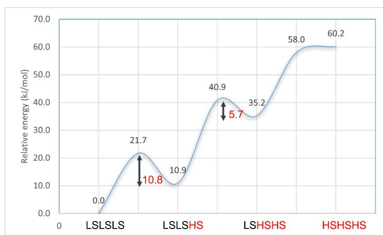
Figure 2. Relative energy (in kJ/mol) for the different spin solutions of the 2D molecular layer deposited on Au(111). The zero-point energies are not included. The activation barriers for the successive spin transitions on cooling are indicated in red.
