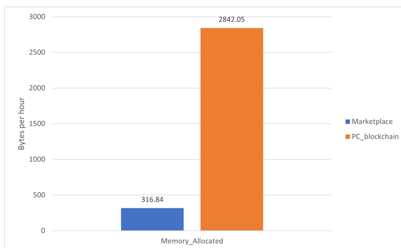
Figure 7. Comparison of the memory allocation metric between the proposed marketplace and an analogue blockchain over a PC.
