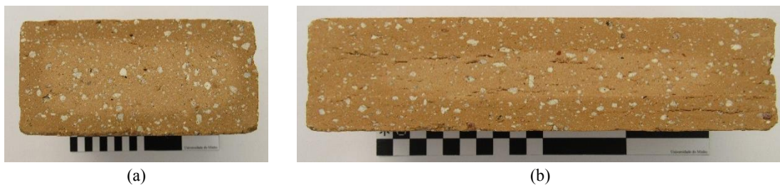
18 Figure 1. Cross-sections of fired-clay brick units: (a) transversal section through the middle plane; (b) 19 longitudinal section through the middle plane.
