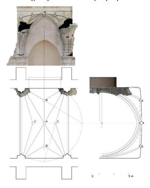
Fig. 17: Geometric framework of a vault based on the orthogonal projections of the scanned *tas-de-charges*
