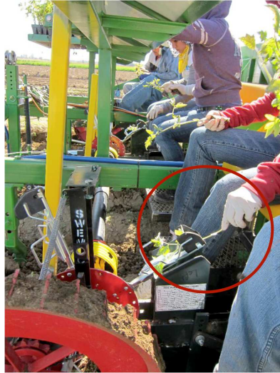
Figure 6. Photograph showing the position of the root ball relative to the fingers of the transplanter. The root ball (held inside the person's hand in the foreground) is typically cantilevered 7-5 m em past the end of the finger.
