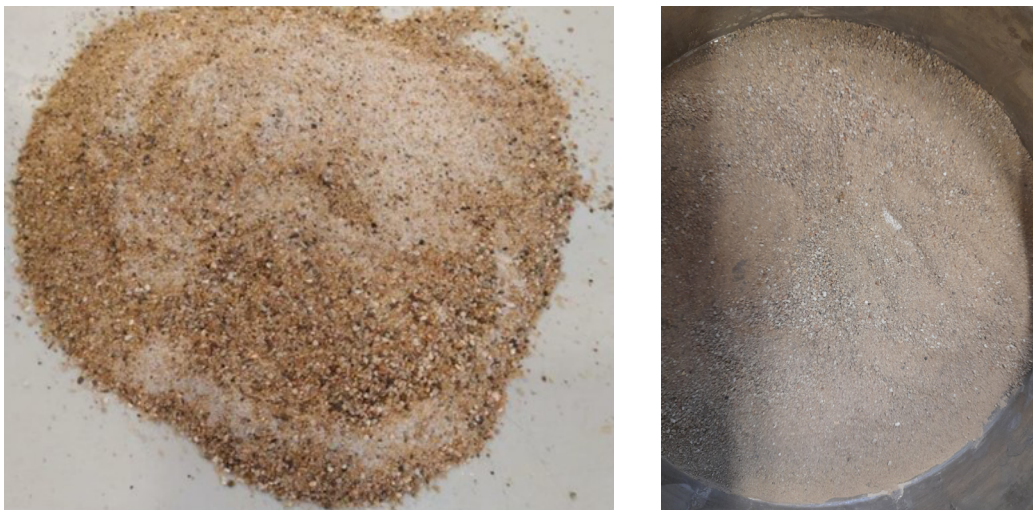
FIGURE 1. Standard sand (left) and demolition and construction waste (right) as fine aggregate.
