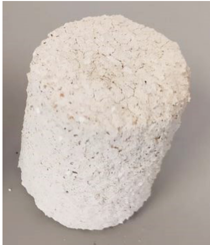
FIGURE 13. Outer appearance of recycled sand mortar after immersion in acid.
