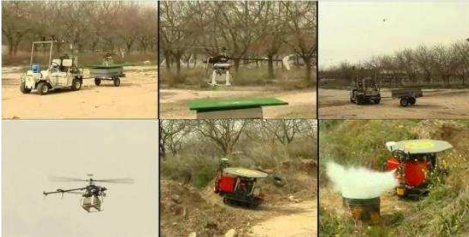
Figure 2.9: Some pictures of the demonstration in the “Alamillo” Park. The goal of the mission is to detect a fire and extinguish it with the collaboration of three robots: ROMEO-4R, HERO2 and AURIGA.
