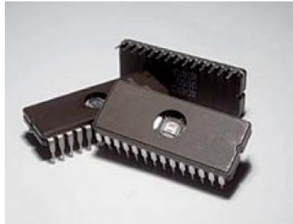
Figure 2.5: Packaged integrated circuit
