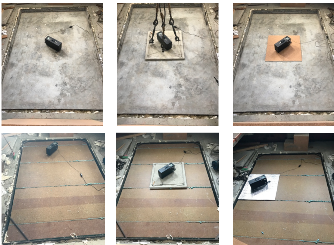
Figure 5. Impact noise measurements (emission room) of homogeneous (H) and non-homogeneous lightweight floor (NH): a-d) uncoated base floor, b-e) floating floor systems, c-f) material placed as floor coverinas.
