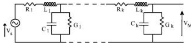
Figure 1-12 : Distributed parameter model of a connection line [37]
