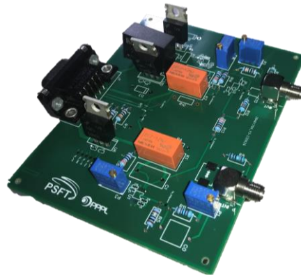
Figure 4-15 : Assembly of through-hole components
