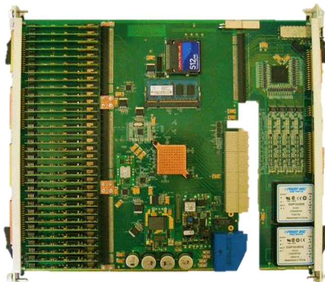
Figure 3-16 : Example of an ATCA-MIMO-ISOL board developed by IPFN [69]
