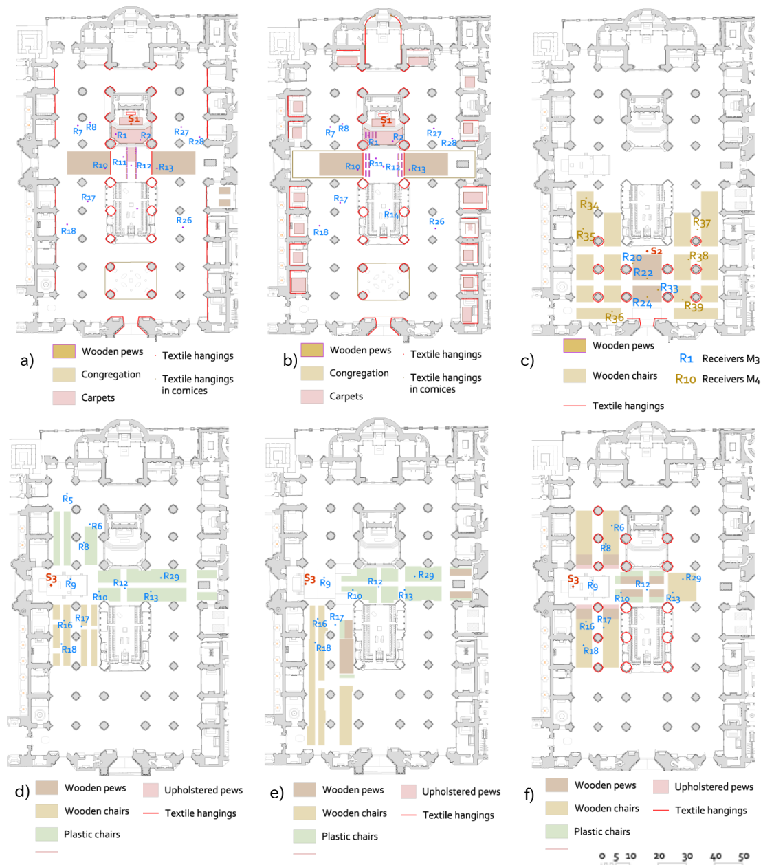
Figure 2. Configurations adopted inside the cathedral of Seville: a) M1; b) M2; c) M3 and M4; d) M5; e) M6; f) M7 and M8.
