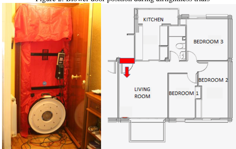
Figure 2: Blower door position during airtightness trials
