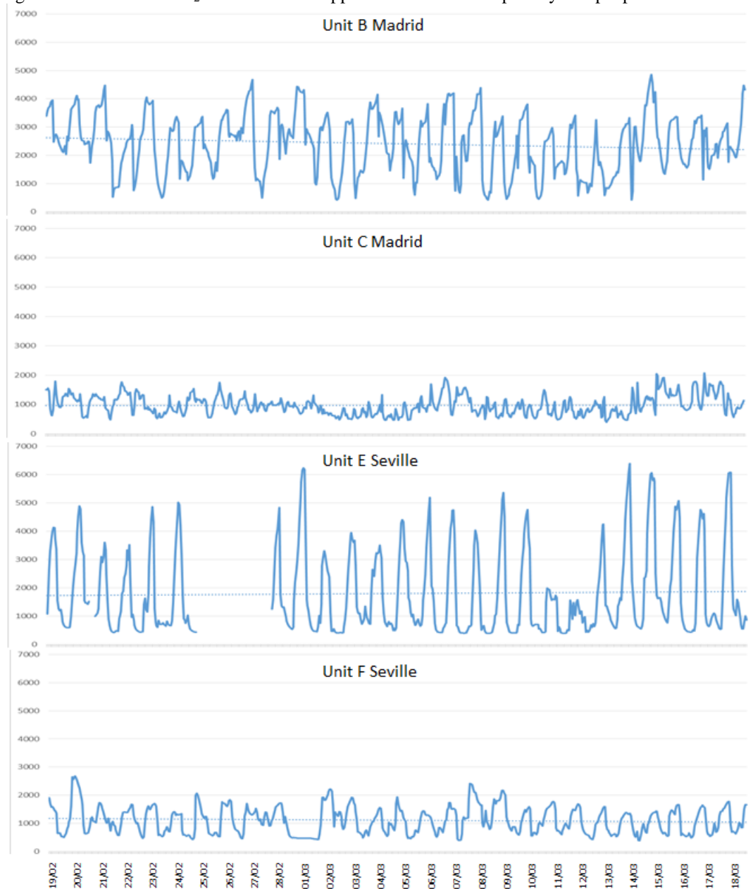
Figure 6: Winter time CO 2 concentration in ppm in bedrooms occupied by two people in selected units
