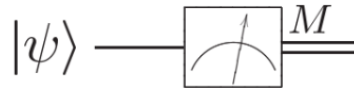
Figure 1.4: Quantum circuit symbol for single qubit measurement, obtained from [1]. The two lines after measurement refer to a bit and not a qubit, since the state has collapsed, with M being the measured state.
