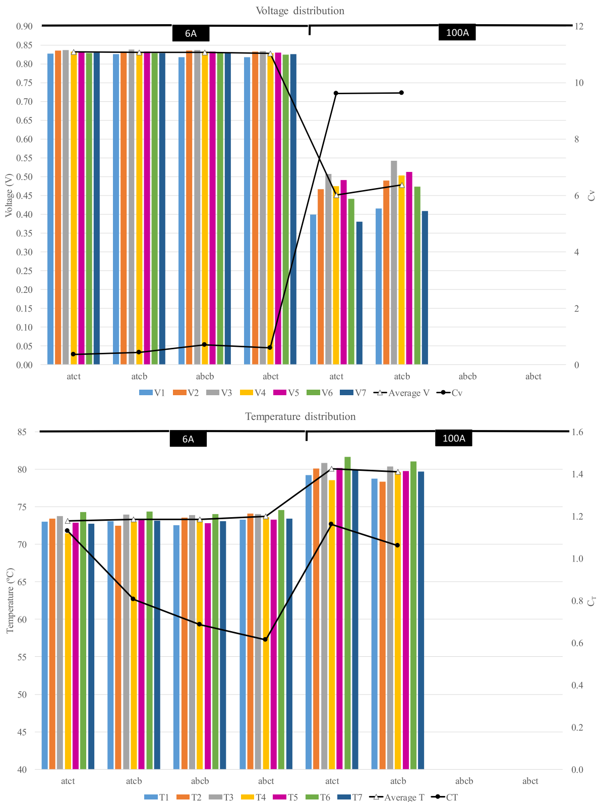
Fig. 11. Voltage (top) and temperature distribution (bottom) at a current density of 0.06 and 1 A/cm 2 .
