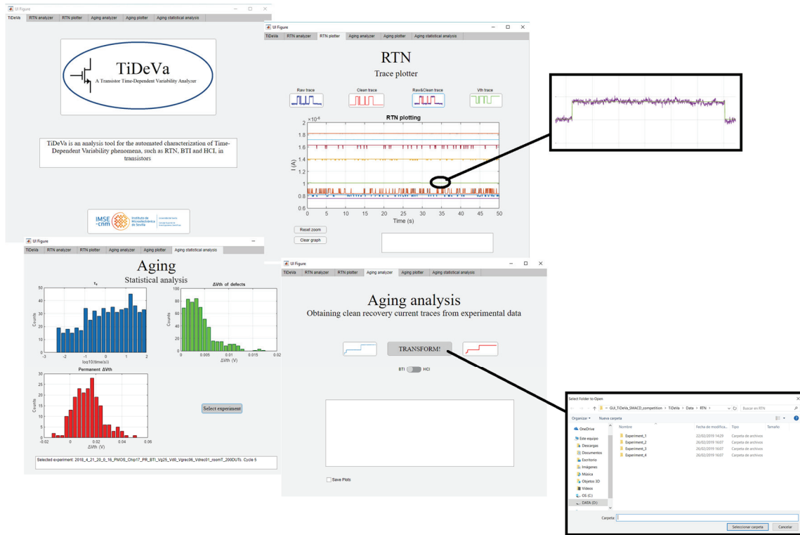
Fig. 11. Some tabs of TiDeVa. The one at the top-left corner is the one to open when the user launches TiDeVa. Then, clockwise, there is the tab for the graphical visualization of the RTN current traces, the tab for the analysis of aging experiments data, and the tab for the visualization of the statistical distributions obtained for the parameters of an aging experiment.
