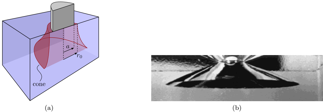
Figure 2: Indentation fracture caused by a flat-ended cylinder: (a) sketch of the indentation test and crack topology; (b) cone-shaped crack obtained with a cylindrical punch in soda-lime glass, adapted from (Lawn, 1998).
