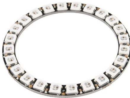
Figura 37: Anillo NeoPixel, 24 LED's – WS2812 RGB [10]
