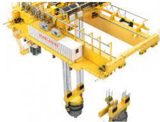
**Figura 3.2** Landle Crane (Puente Grúa)[2].
