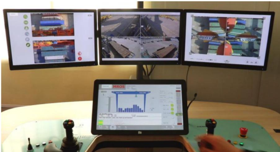
Figura 3.11 RCOS - Remote Control Operation System[2].
