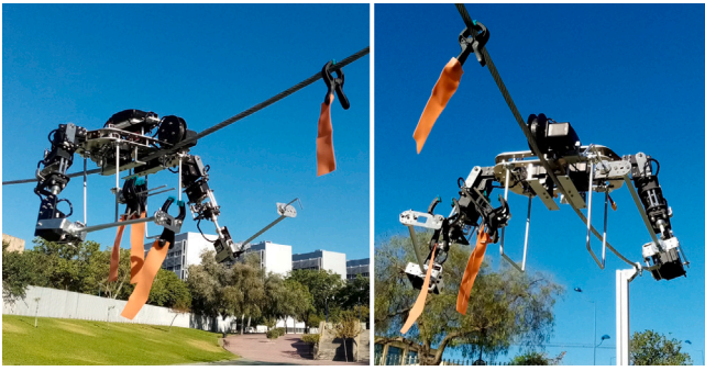
Fig. 1. Lightweight and compliant, anthropomorphic dual-arm rolling robot installing clip-type bird flight diverters on a power line.
