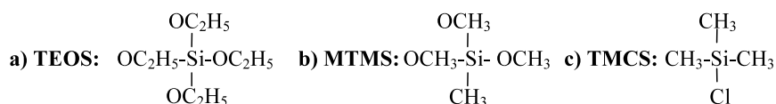
Fig. 1. Schematic representation of the molecules involved in the composition of the samples studied: (a) TEOS; (b) MTMS; and (c) TMCS.
