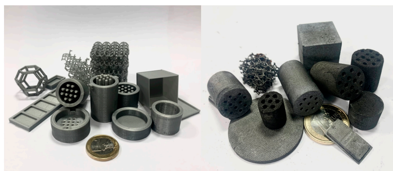
Figure 1. Examples of prepared PLA molds (left) and carbon monolithic devices (right).
