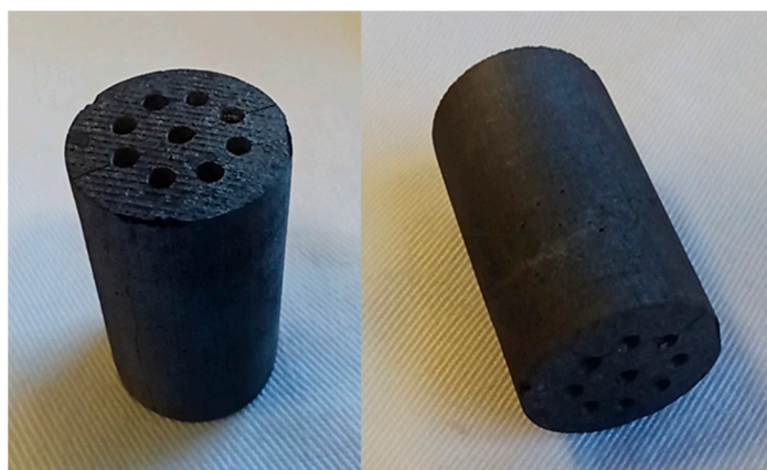
Figure 7. Monolith used in the catalytic test.
