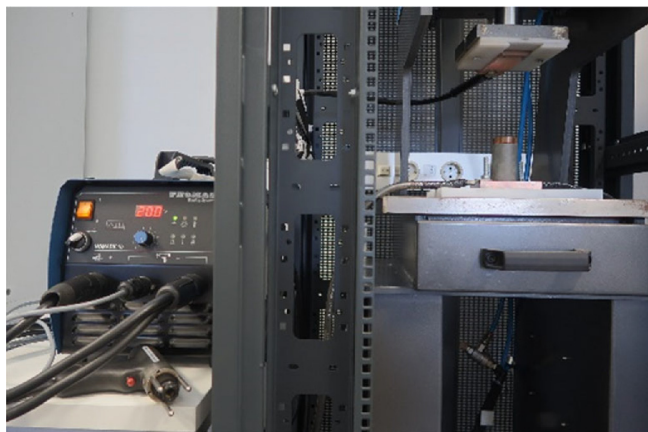
Fig. 1. Stud welding equipment and pneumatic press used in the experiments.
