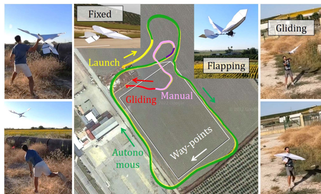
Fig. 1. Hybrid fixed-flapping wing aerial robot conducting an autonomous operation in outdoors consisting of following a trajectory defined by four way-points. The platform is hand launched and safely captured by a human.
