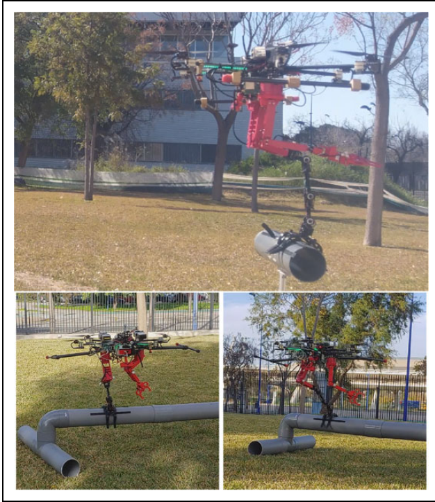
Figure 22. Test of the docking tool system in real environment.
