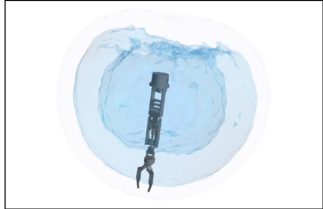
Figure 11. Kinematic reachability of the robotic arm with the gripper of 2 DoFs. DoF: degree of freedom.
