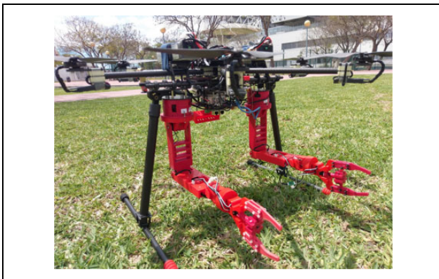
Figure 19. UAV on the ground with the two robotic arms with the gripper tool. UAV: unmanned aerial vehicle.
