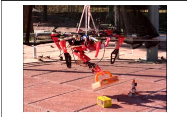
Figure 18. Aerial robot with single manipulator.
